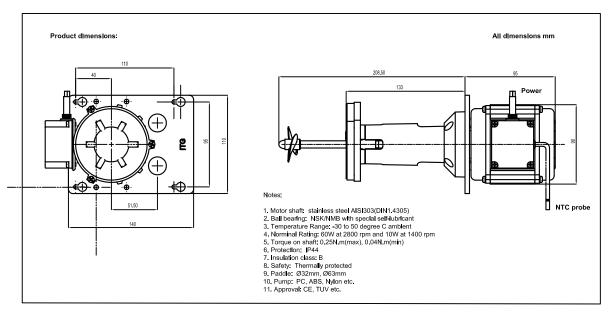
Brushless DC motors from ITG are electronically commutated (EC) motors. They are very high efficiency(>73%) electric motors and maintain a high efficiency level at part speed.
